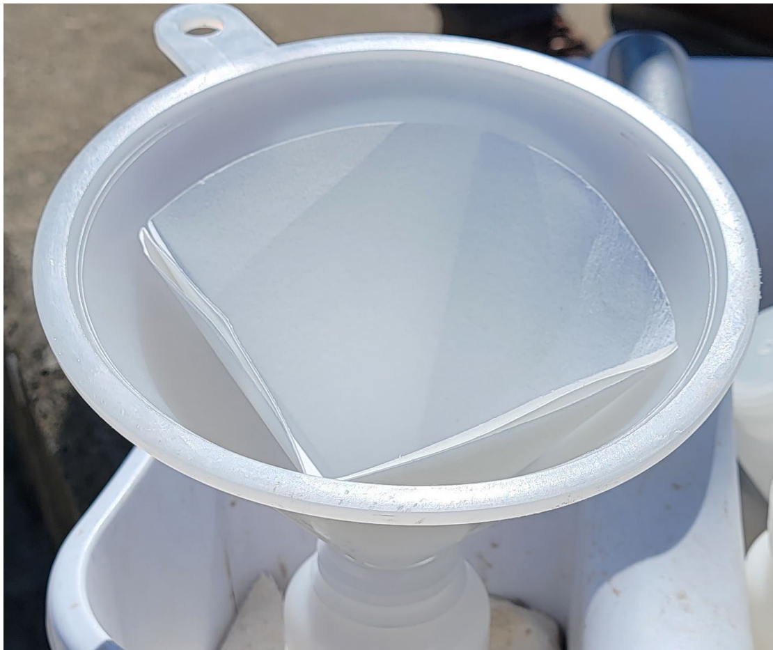
Figure 2. Image of a large diameter filter paper that has been folded and placed inside a plastic funnel for sample collection.
